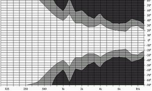
Isobar diagram E12 horizontal, horizontal setup with the horn rotated
